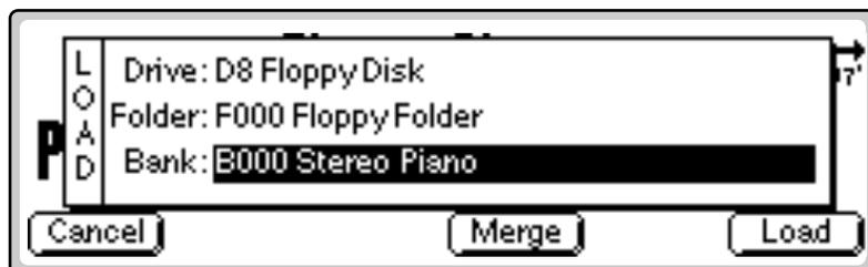
2. **Select the Drive.** (If you have a hard disk or CD-ROM connected otherwise skip this step.) Using the Arrow cursor buttons, move the cursor to the Drive field and select, "D8 Floppy Disk".
