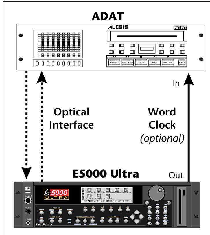
*This diagram shows how to connect an E5000 to an Alesis ADAT™ using the optional ADAT interface card. The Word Clock connection is optional, but provides a slightly more stable clock source.*
