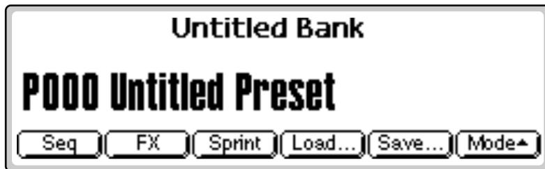
If you had the ROM bank added, you could select presets immediately using the Data Entry Control, INC/DEC buttons, Left/Right cursor buttons or the numeric keypad to change presets. Without the ROM bank installed, you must load a bank into the unit. See the next page for instructions.
