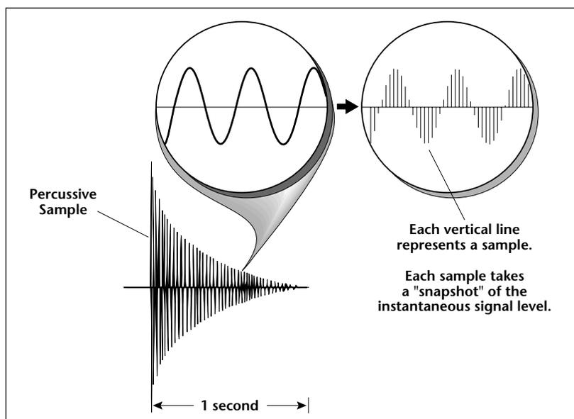
Conceptually, sampling is like a tape recorder. However, the recording process is different since the E5000 records into its computer memory digitally. Samples can be loaded via removable-media hard disk, magneto-optical disk or CD-ROM using the SCSI interface. They can be sampled through the analog inputs or the AES/EBU digital interface, or even through the MIDI interface using MIDI Sample Dump or SMDI.
