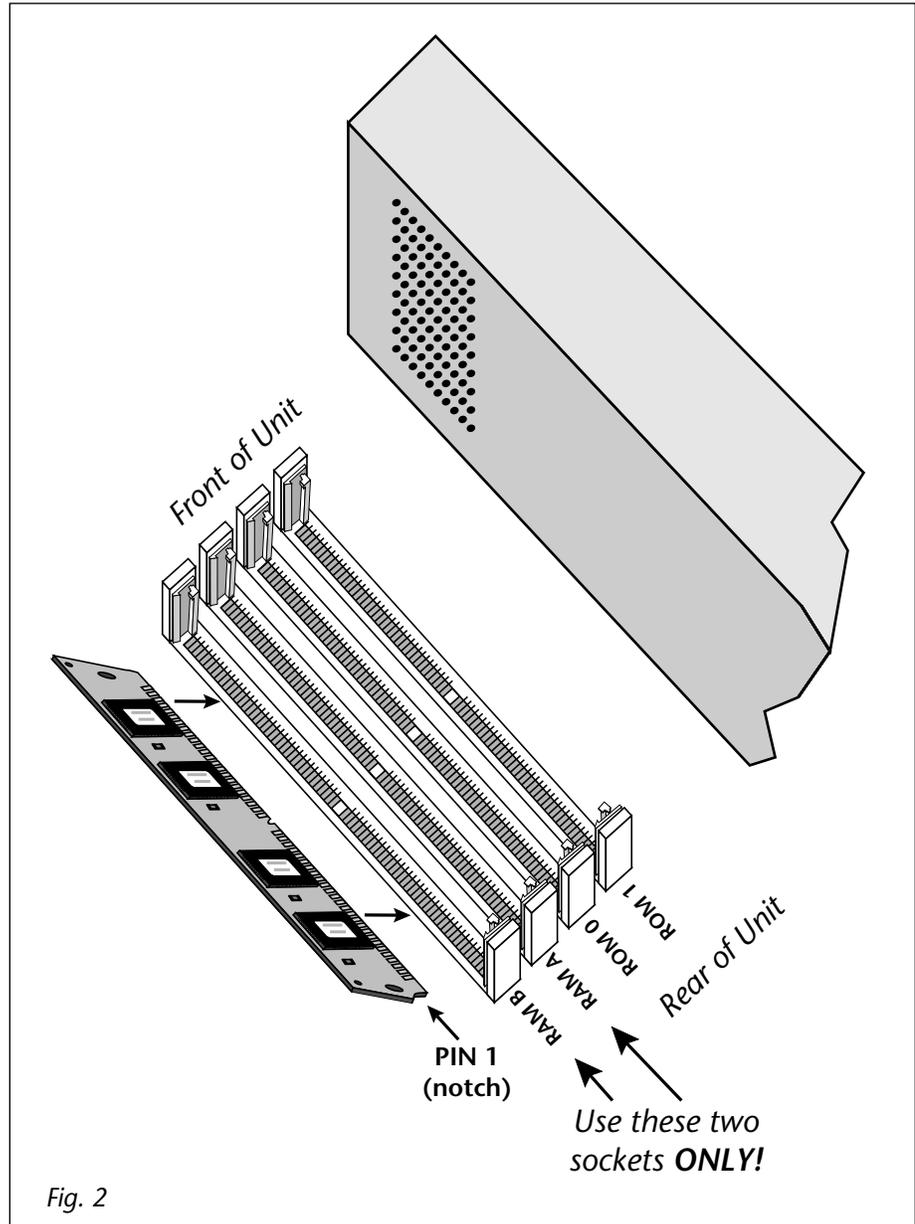
7. While applying a slight downward pressure on the top of the SIMM to keep it from popping out of the socket, tilt the SIMM board into a vertical position as shown in figure 3. You should hear an audible click. Make sure both sides of the silver tabs have latched.
